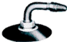
**TRJS2** Small rubber based metal stem valve for industrial applications. This valve fits .445"/.461" diameter rim hole and can be used with liquid fill. Valve is bent at 70° and supplied with a washer and nut.
